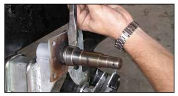
1. Remove hub unit from spindle Use a large sized and sharpened chisel to split open wear sleeve. Try not to chisel into the spindle; if possible, only chisel into the wear sleeve. Wear sleeve should spring open.
