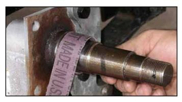
3. Use various "grit" emery or crocus cloth to remove any burs on the spindle that may have occurred from the chisel. Start with a coarse grade emery or crocus cloth working your way towards a fine grade. Example: Start with 80 grit, then use 120-160 grit, then use 240-320 grit emery or crocus cloth. Purpose is to repair any damage created on the 0-ring seal groove section of the spindle.
