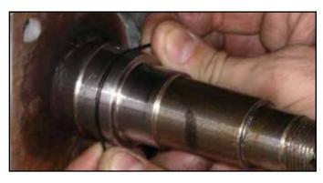
4. Once any and all burs and sharps have been removed, replace the old spindle/wear sleeve O-ring with a new O-ring; lightly lubricate the O-ring prior to assembly. Inspect O-ring for any damage prior to assembly over the spindle. Ensure O-ring is fully seated inside of the seal groove.
