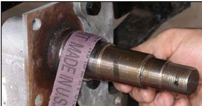
**3.** Use various "grit" emery or crocus cloth to remove any burrs on the spindle that may have occurred from the chisel. Start with a coarse grade emery or crocus cloth working your way towards a fine grade. Example: Start with 80 grit, then use 120-160 grit, then use 240-320 grit emery or crocus cloth. Purpose is to repair any damage created on the O-ring seal groove section of the spindle.
