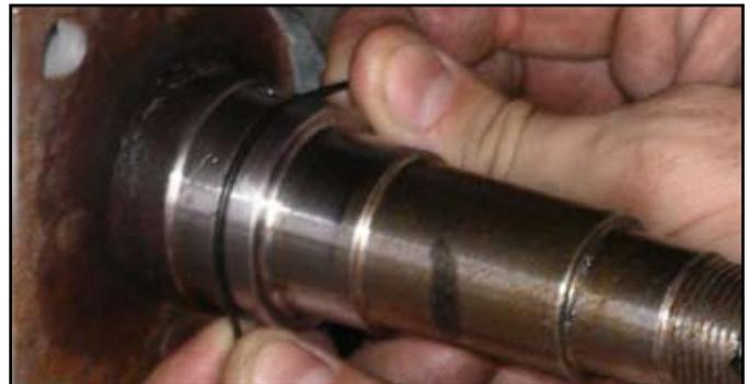
**4.** Once any and all burrs and sharps have been removed, replace the old spindle/wear sleeve O-ring with a new O-ring; lightly lubricate the O-ring prior to assembly. Inspect O-ring for any damage prior to assembly over the spindle. Ensure O-ring is fully seated inside of the seal groove.
