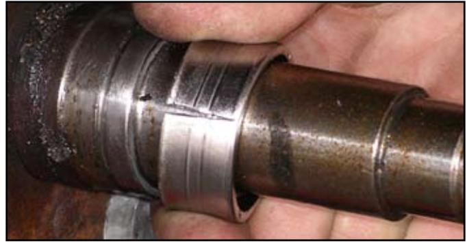
**2.** Once the press-fit bond of the wear sleeve has been broken, remove the old wear sleeve from the spindle
