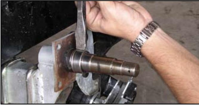
**1.** Remove hub unit from spindle Use a large sized and sharpened chisel to split open wear sleeve. Try not to chisel into the spindle; if possible, only chisel into the wear sleeve. Wear sleeve should spring open.
